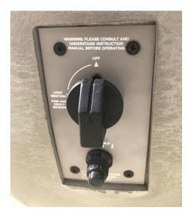
Step #8 - Turn knob counter-clockwise to "low ignition" location.
